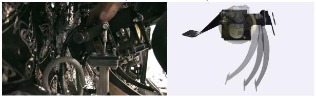
• Once all clearances are checked bolt the unit in place, via the dash mount and fire wall mount.
