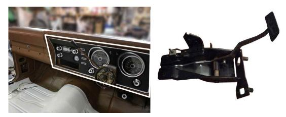
Mock RRS under dash assembly in, check for wiper clearance, the rear of the pedal are free from wires, hoses and pedal travel has adequate clearance
