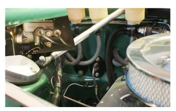
RRS blanked off the two brake warning switch positions
