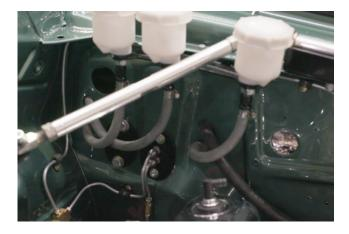
• Mount reservoir holder (insure higher than top of master cylinder)
